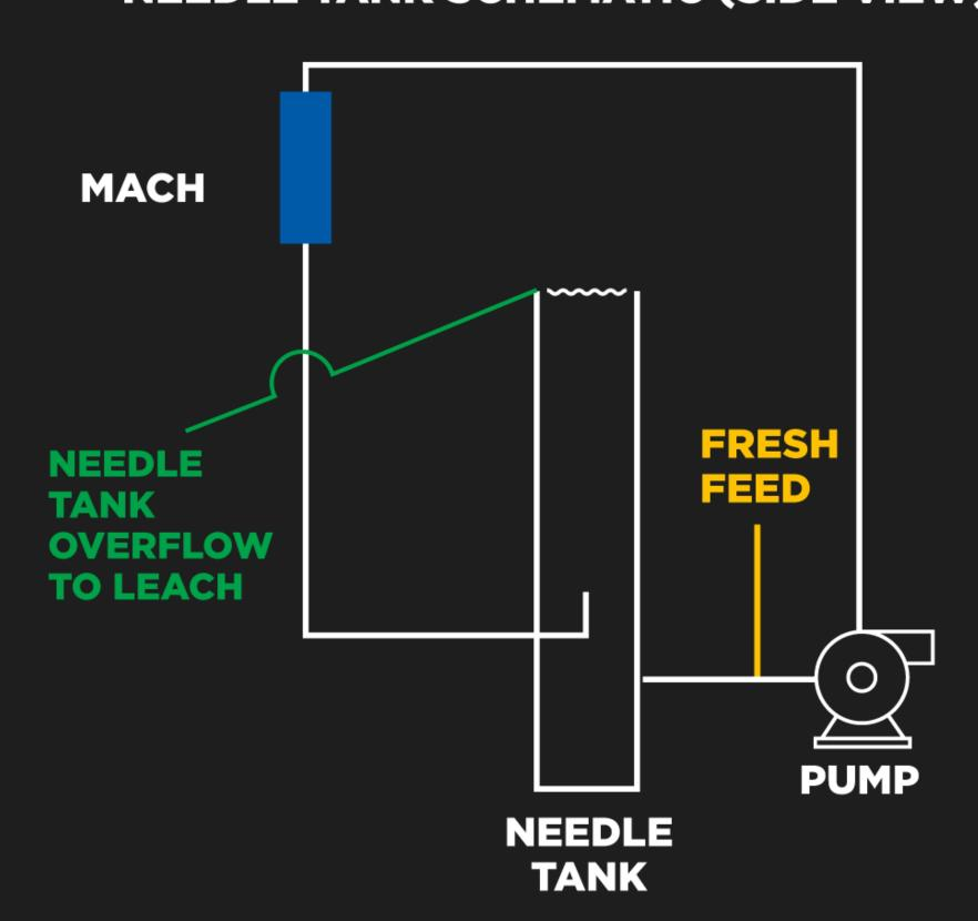
The MACH REACTOR™ can be installed in-line with the flow into the first Leach Tank or on Tank Recycle (preferred).
