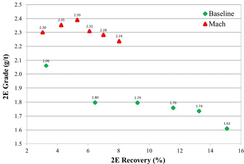
Figure 3 – Grade vs recovery for Mintek pilot plant work
