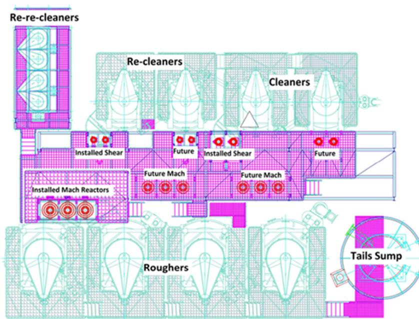
Figure 6 – General arrangement drawing showing the installation of all of the planned reactors with respect to the flotation cells
