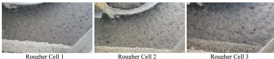
Figure 7 – Photographs of the first three rougher cells with the Mach Reactors online and the blowers offline
