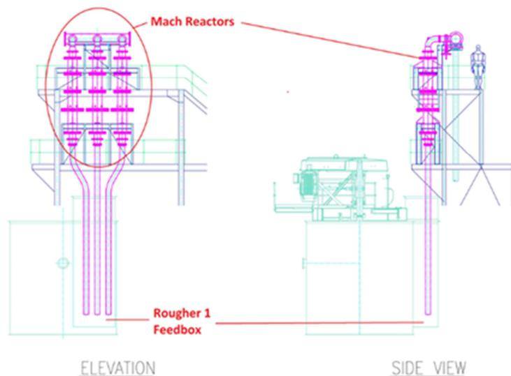
Figure 5 – General arrangement drawing showing the installation of the Mach Reactors on the first rougher cell
