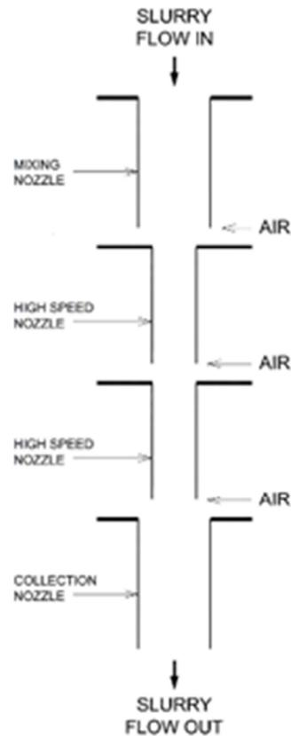
Figure 1 – Schematic of Mach Reactor internal design
