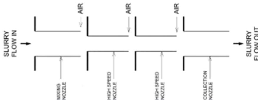
**Figure 3** Schematic of Mach reactor (Singh, 2016).
