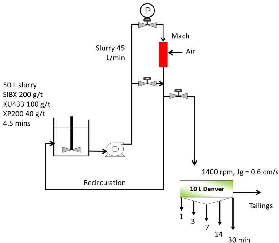
**Figure 4** Experimental setup for flotation tests.
